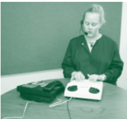
A typical relay operator transmits a call using a TTY and a voice telephone.
